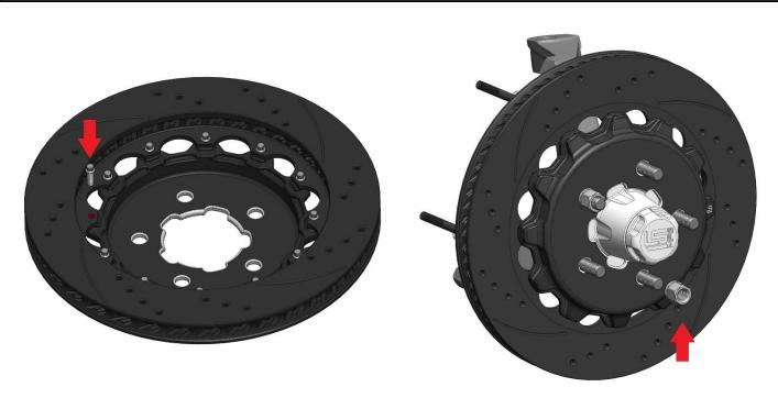
Arrange the rotor and hat in the position shown ensuring the arrow noting rotation direction is correct for its position on the vehicle. Start the first few threads of all 12 of the ¼-20 12-point bolts. Using an alternating sequence, apply red Loctite® 271 to the threads, and torque to **155 in-lbs**. The rotor can be installed on the hub at this time using two lug nuts to hold the hat flat against the hub.
