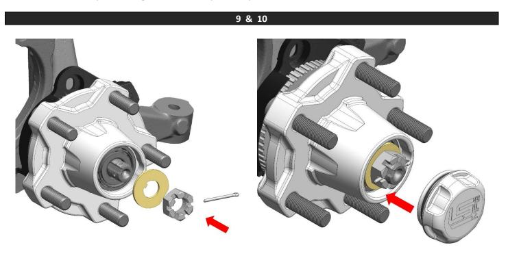
You can now install the hub onto the spindle, then pack the outer bearing (A3) with grease and install under the factory washer, castle nut, and supplied cotter pin. Install the machined dust cap as shown.
