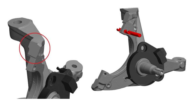
Sand the trimmed surfaces smooth. Any sharp tips left over must be sanded flat to avoid contact with the new caliper radial bracket. Drill the original caliper mounting bolt holes with a 7/16 drill bit (not included). Check the drilled area for burs and sand smooth if necessary.
