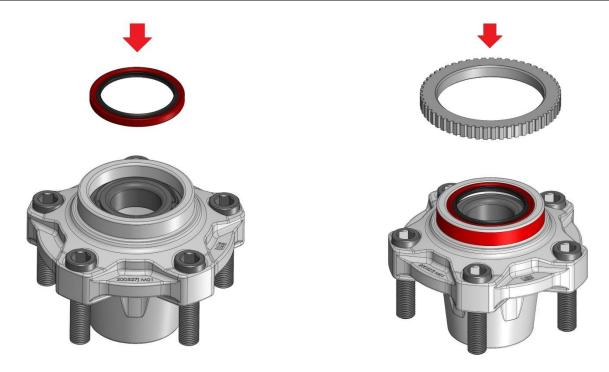
Pack the large inner bearing (A5) with high temperature disc brake bearing grease and install into the back side of the hub. The inner seal can then be pressed in or lightly tapped in with a hammer by circling the perimeter. **If your truck has front wheel ABS**, remove the reluctor ring from the stock rotor and install it onto the hub. The ABS pickup magnet will be remounted to the spindle using the bolt hole it previously used on the dust shield.
