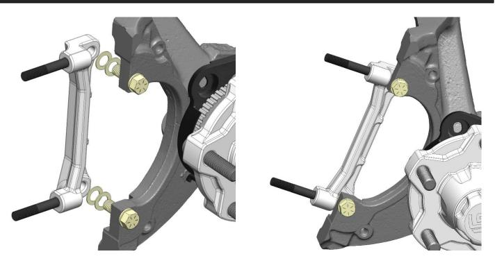
The radial bracket can temporarily be installed at this time using the supplied bolts and two .750x.438x.030 shim washers between the bracket and spindle. It is not necessary to torque them at this time.
